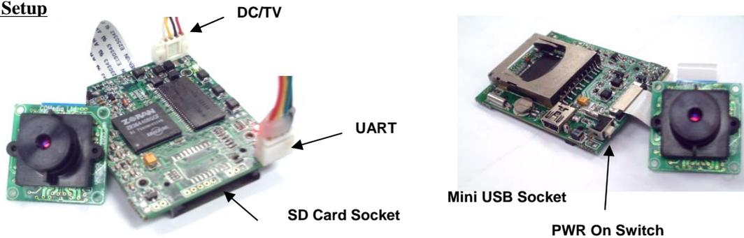
1. Plug in the 4pin connector of UART adapter cable to the UART socket
